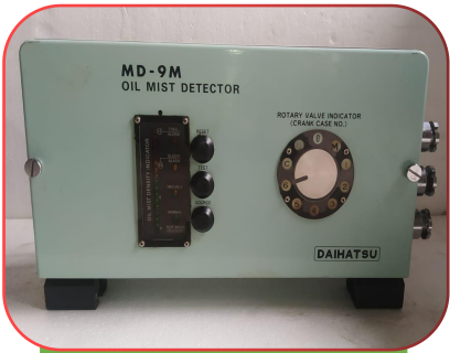
Oil Mist Detector for Engines
